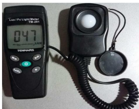
Slika 1. Mjerni instrument TENMARS Lux/Fc Light Meter TM-201
