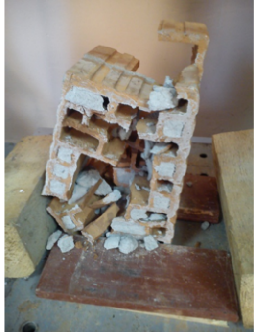
Figure 4.4: Tensional failure parallel to bedjoints (Penava, 2012)
