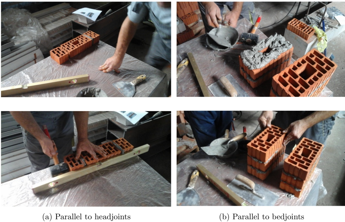
Figure 4.3: Preparation of masonry triplet tests (Penava, 2012)
