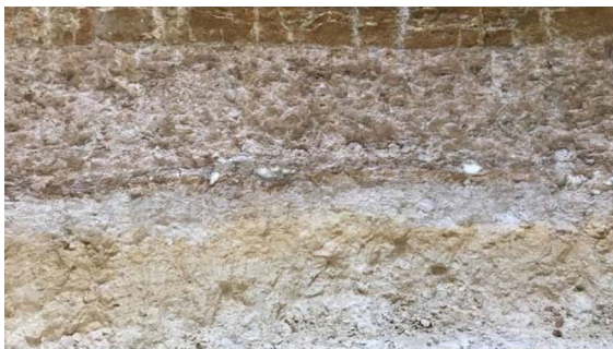
Fig. 4 From the top: Midra shale layer, Khor limestone layer, and Rus calcareous layer
