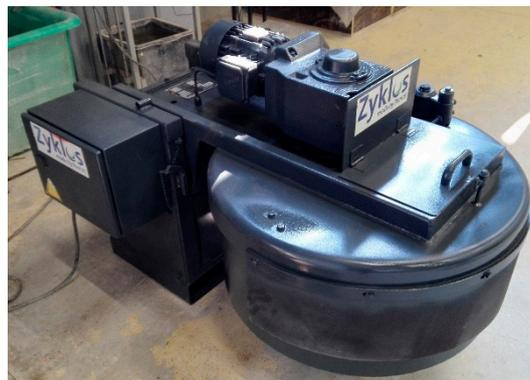
**Figure 3.** Pan mixer (50 L capacity).
