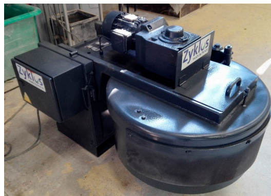
Figure 3. Pan mixer (50 L capacity).
