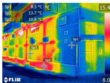
Figure 2. An example of highly-visible structural elements as well as a heated and an unheated space.
