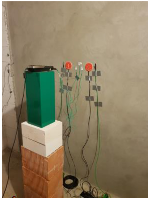
Figure 5: HFM method and TBM.
