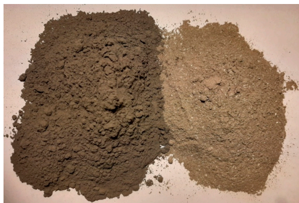
Figure 1. The appearance of cement (left) and CWA (right).
