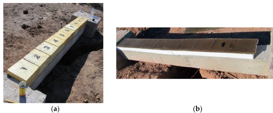
Figure 12. RC columns reinforced with: (a) polyurethane bricks [15,16] and (b) resin panels and insulation layer [22]. Copyright permission obtained from authors.
