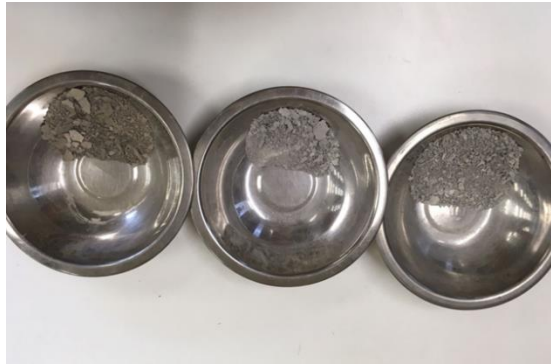
Figure 8. Total residues of scaling material of mortar mixture M2 (left), mortar mixture M1 (in the middle) and reference mortar mixture R (right)
