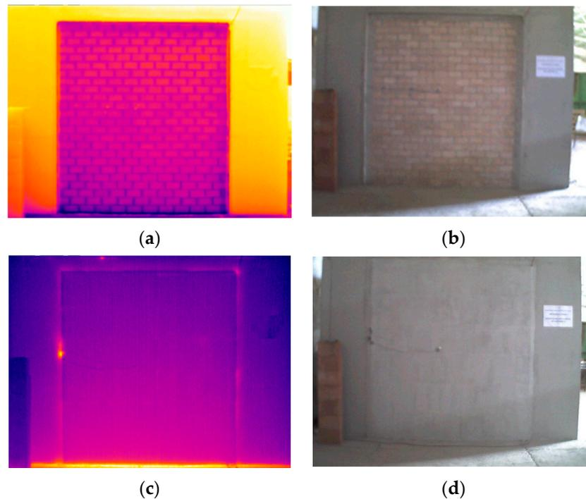
**Figure 8.** IR thermography (a) IRT image during a cooling period (autumn/summer), (b) wall without thermal insulation, (c) IRT image during cooling period (winter), (d) wall insulated with mineral wool.
