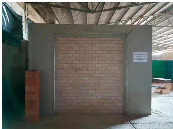
**Figure 5.** Wall made of RBC-EP masonry block—without isolation.
