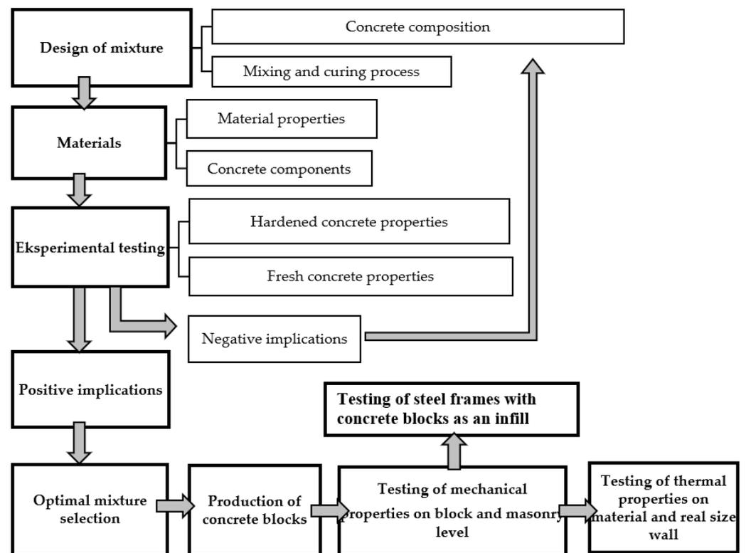
Figure 2. Flowchart of the experimental investigation.
