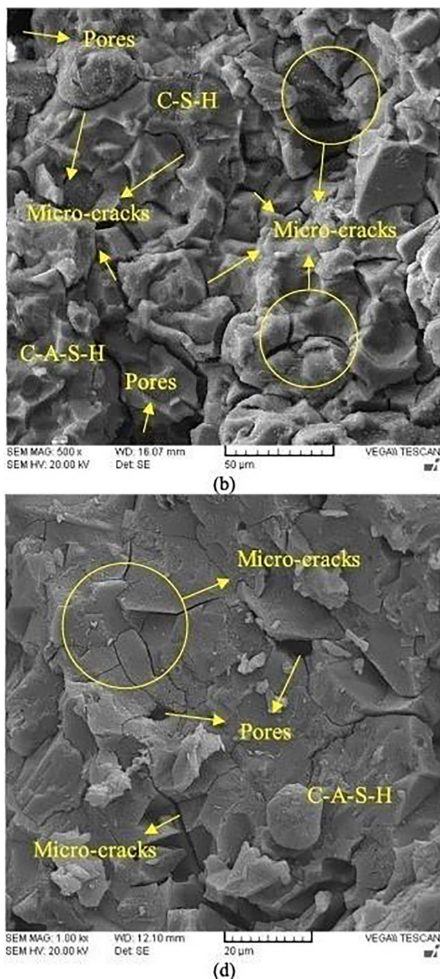
Fig. 13. Influence of GP content on microstructure (a) 100%SL (b) 70%SL30%GP (reused with permission (Shoaei et al., 2020)).
