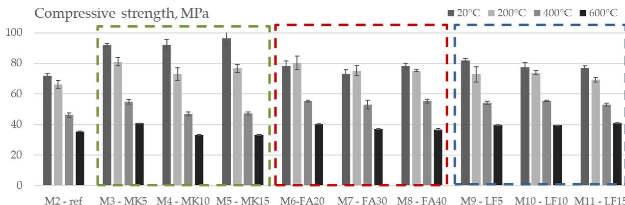
Figure 9. Compressive strength vs. temperature of tested mixes.
