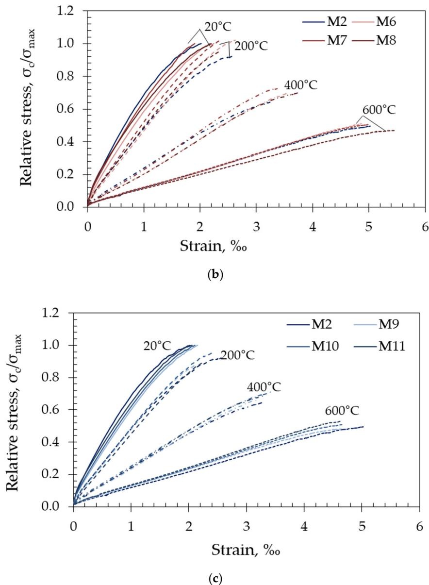
**Figure 8.** Normalised stress–strain curves for (a) metakaolin based (M3–M5), (b) fly-ash based (M6–M8) and (c) limestone based (M9–M11) in relation to the reference mixture (M2) as a function of temperature.
