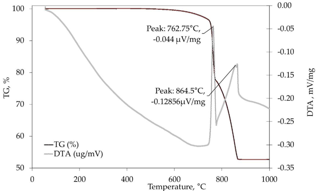
**Figure 2.** TG/DTA graph of dolomite aggregates.
