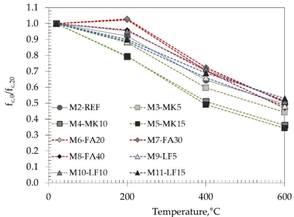
Figure 10. Normalized values of compressive strength vs. temperature.
