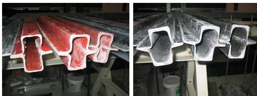
Figure 6. Testing beam samples from GFRP and RGFRP
