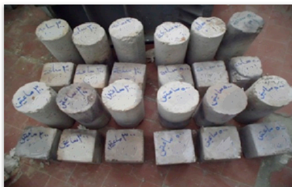
Figure 5. Shapes of specimens after heating.
