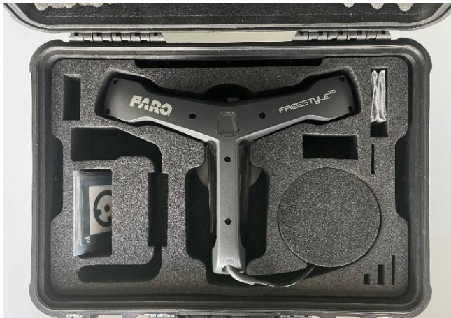
Slika 2. FARO Freestyle 3D laserski skener
