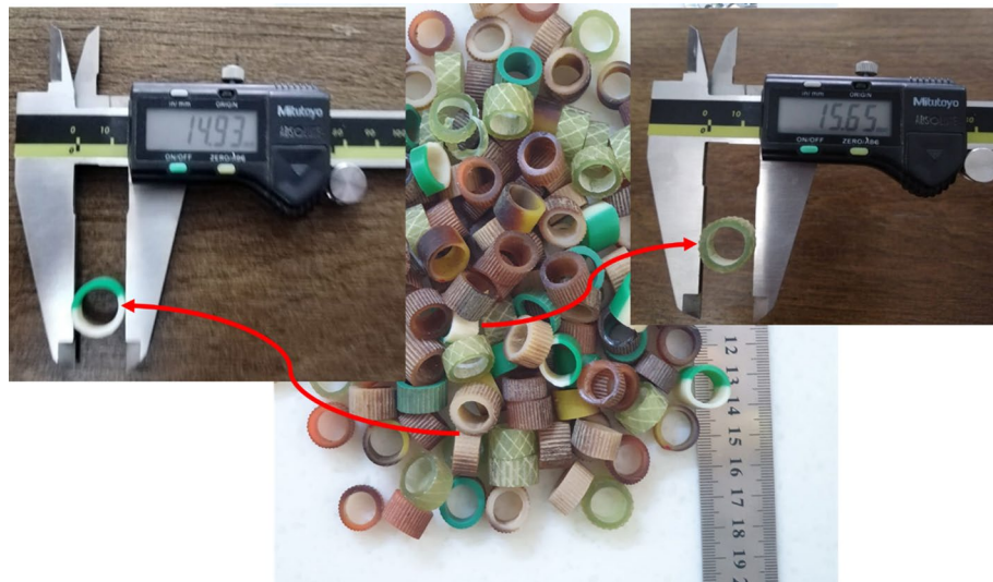
Figure 9. Lightweight waste plastic water hose manually cut using special scissors.
