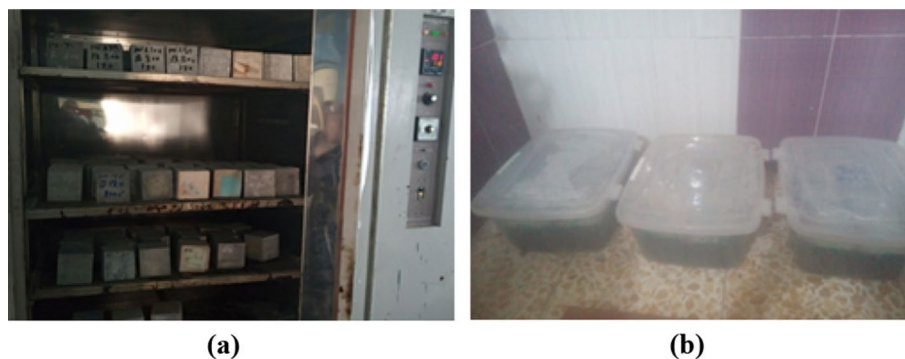
Figure 12. (a) Cubes exposure to evaluated temperature; (b) cubes immersed in water containing 10% MgSO_4 of water weight.
