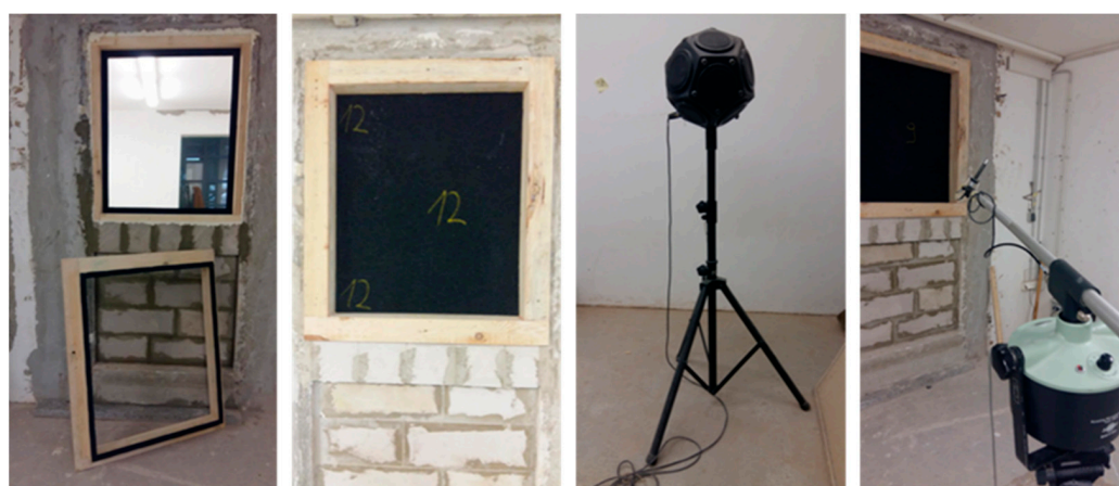
Figure 7. Airborne sound insulation index test setup.
