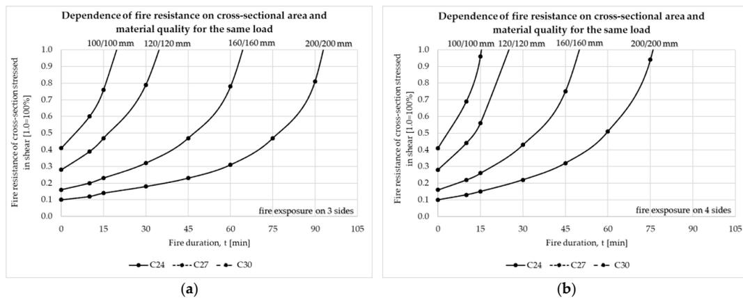
**Figure 7.** Graphical representation of the fire resistance of the cross-sectional area (element) depending on the cross-sectional area and strength class: (a) Fire resistance for a cross-section subjected to shear stress when the fire acts on three sides of the cross-section; (b) Fire resistance for a cross-section subjected to shear stress when the fire acts on four sides of the cross-section.
