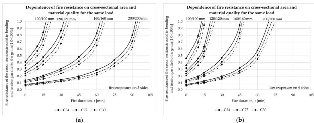
**Figure 9.** Graphical representation of the fire resistance of the cross-sectional area (element) depending on the cross-sectional area and strength class: (a) Fire resistance for a cross-section subjected to bending and tension parallel to the grain when the fire acts on three sides of the cross-section; (b) Fire resistance for a cross-section subjected to bending and tension parallel to the grain when the fire acts on four sides of the cross-section.
