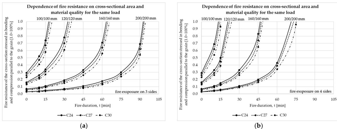
**Figure 10.** Graphical representation of the fire resistance of the cross-sectional area (element) depending on the cross-sectional area and strength class: (a) Fire resistance for a cross-section subjected to bending and compression parallel to the grain when the fire acts on three sides of the cross-section; (b) Fire resistance for a cross-section subjected to bending and compression parallel to the grain when the fire acts on four sides of the cross-section.
