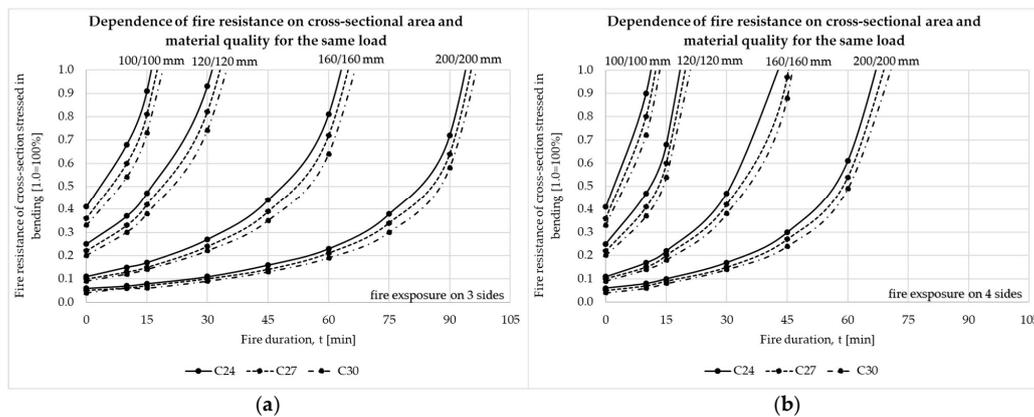
**Figure 8.** Graphical representation of the fire resistance of the cross-sectional area (element) depending on the cross-sectional area and strength class: (a) Fire resistance for a cross-section subjected to bending when the fire acts on three sides of the cross-section; (b) Fire resistance for a cross-section subjected to bending when the fire acts on four sides of the cross-section.
