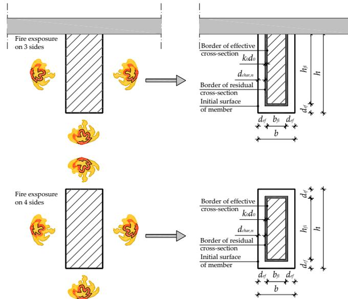
Figure 2. Reduced cross-section method.
