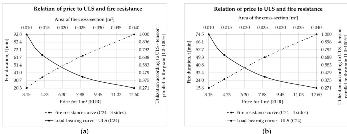
**Figure 11.** Display of price depending on the limit state of load-bearing capacity (tension parallel to the grain) and fire resistance: (a) Cross-section (element) exposed to fire on three sides; (b) Cross-section (element) exposed to fire on four sides.
