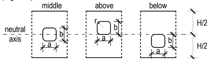
Figure 4 Dimensions for eccentrically positioned openings [18]
