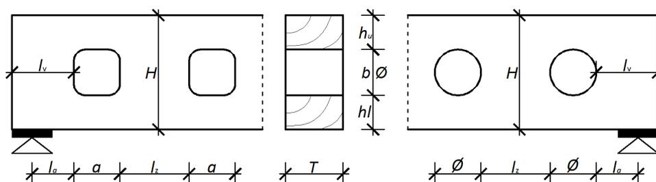
**Figure 9 Dimensions of the girder with openings [25]**
