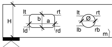
Figure 7 Opening dimensions and crack locations [1]
