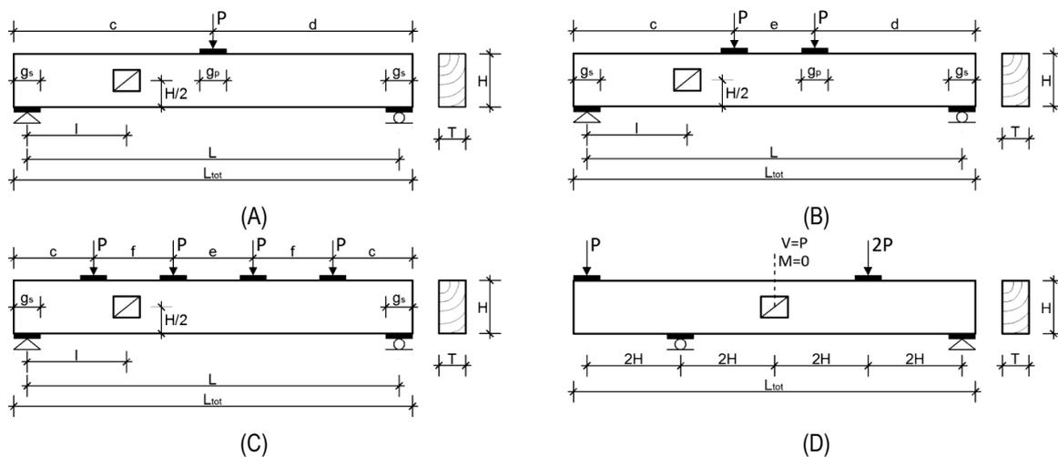
Figure 5 Test setups for straight beams [1, 20]
