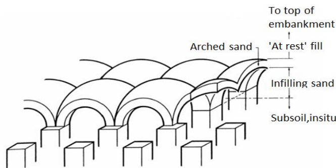
Figure 6 The Hewlett and Randolph method for modeling a reinforced earth structure over piles [13]
