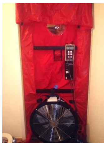
Figure 3 Blower door fan with manometer DG-700 [10]
