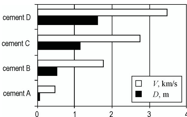
**Figure 8** Length of bonded samples D and speed of ultrasound waves V
