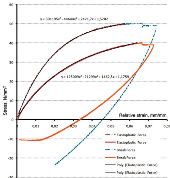
Figure 16 Idealised stress/strain diagram with a cubic curve
