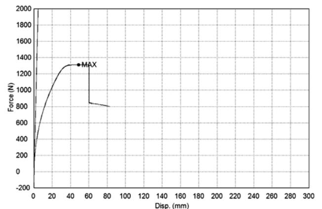
Figure 10 Breaking of a single strap sample
