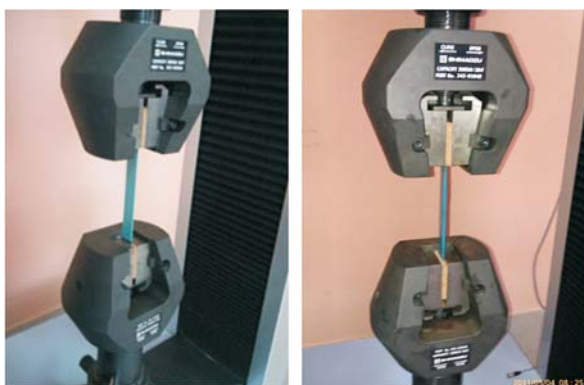
Figure 2 Testing machine and multiple strap samples
