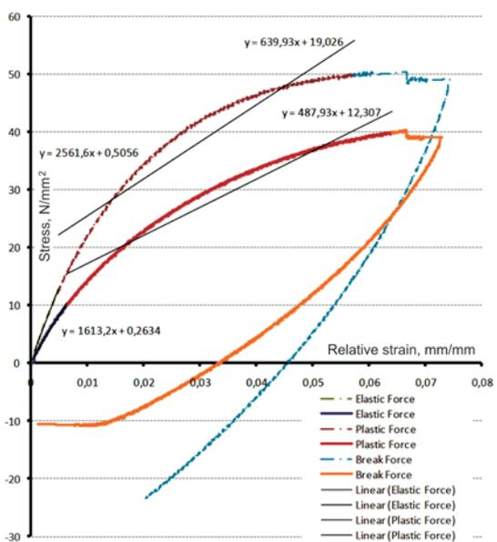
Figure 13 Bilinear idealisation of the stress/strain diagram
