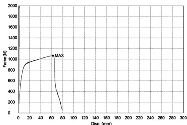
Figure 8 Breaking of a triple strap sample
