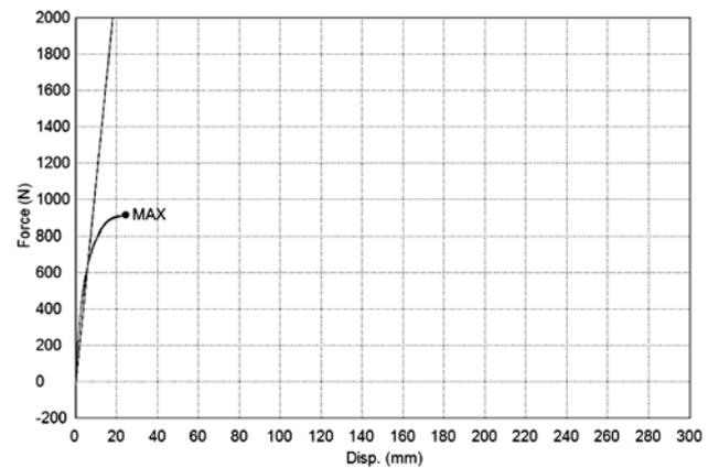
Slika 9 Breaking of a triple strap sample
