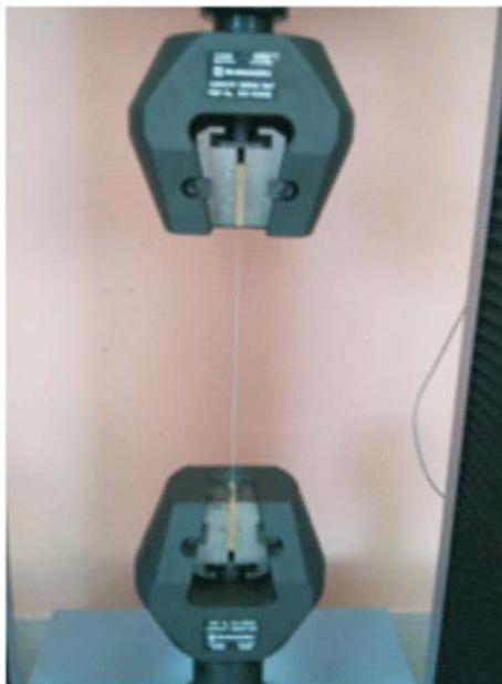
Figure 1 Testing machine and single strap sample
