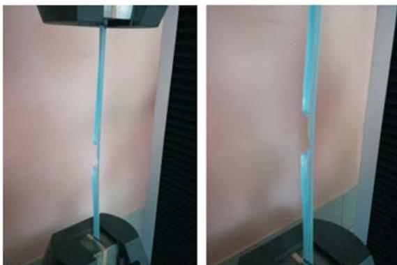
Figure 3 Breaking of the single strap sample
