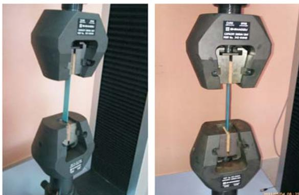
Figure 2 Testing machine and multiple strap samples
