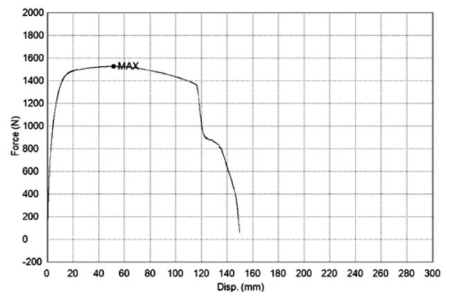
Slika 11 Breaking of a six strap sample
