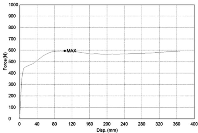
Figure 6 Breaking of a single strap sample
