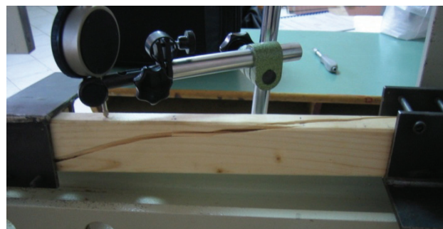
Figure 8 Failure by separation and breaking of fibres
