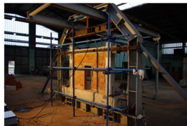
Fig. 2 Infilled frames tested by (Penava 2012)
