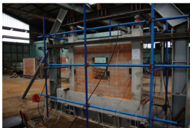
Fig. 2 Infilled frames tested by (Penava 2012)
