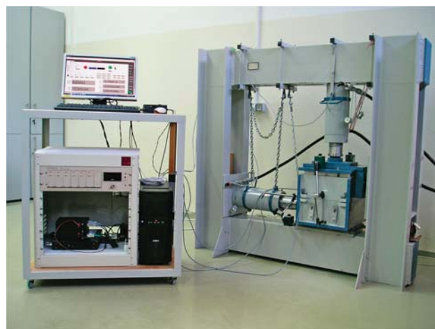
Figure 5: Large direct shear testing (LDST) developed at the Faculty of Mining, Geology and Petroleum Engineering
