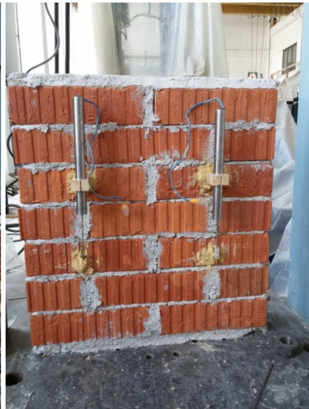
(c) LVDT placement
