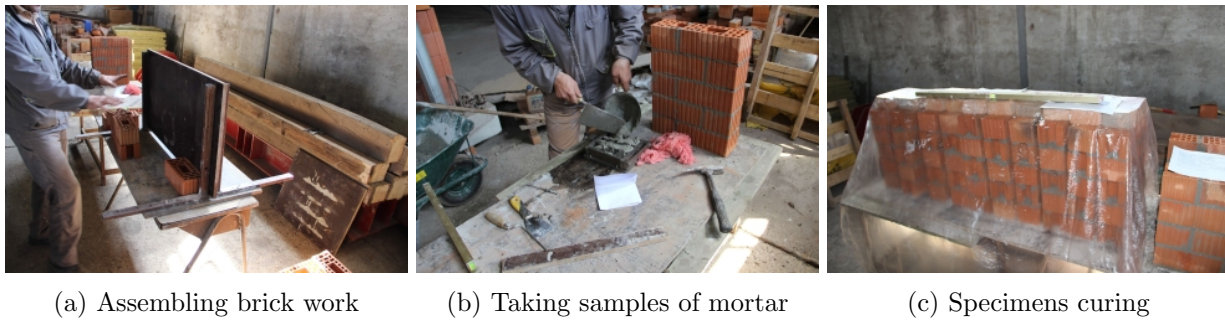
Figure 4.10: URM wall OoP bend test preparation of samples
