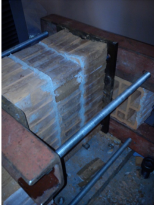
Figure 4.4: Tensional failure parallel to bedjoints (Penava, 2012)
