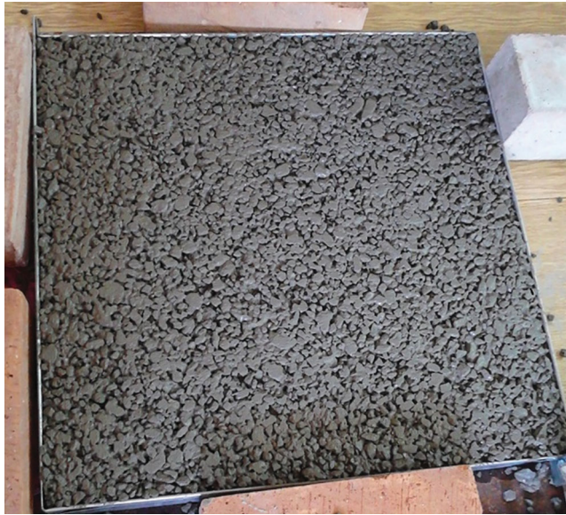
Figure 3. Pervious concrete slab for sound spectral analyses.
