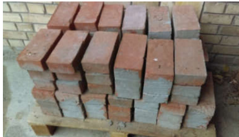
Figure 1. Wall specimens for the initial shear strength.
