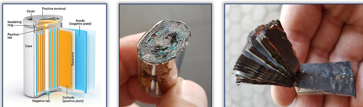
Figure 5. Construction and interior design of a 18650 cylindrical battery
