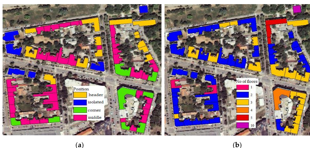
Figure 7. Characteristic block of buildings from the database: (a) position of the building in the block, (b) number of floors.
