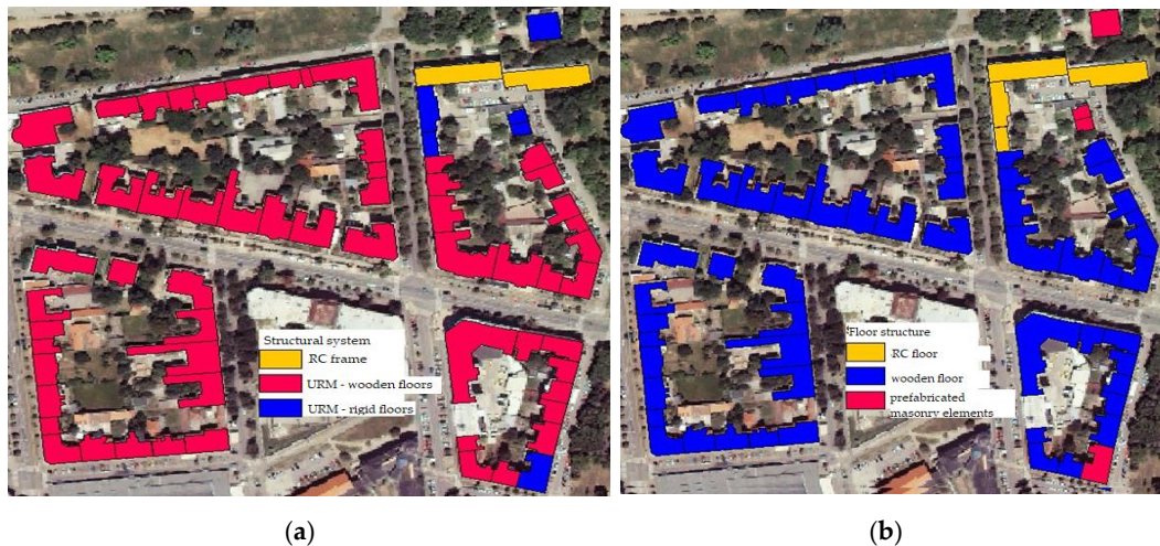
Figure 5. Characteristic block of buildings from the database: (a) structural system, (b) floor structure.
