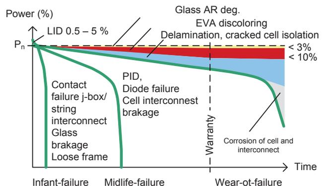
Figure 5. Causes of failure on PV panels, [6]
