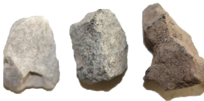
Figure 1. The appearance of the aggregate grain: dolomite, diabase and steel slag.
