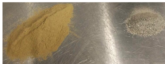
Figure 5. The appearance of used clogging agent: silt and sand.
