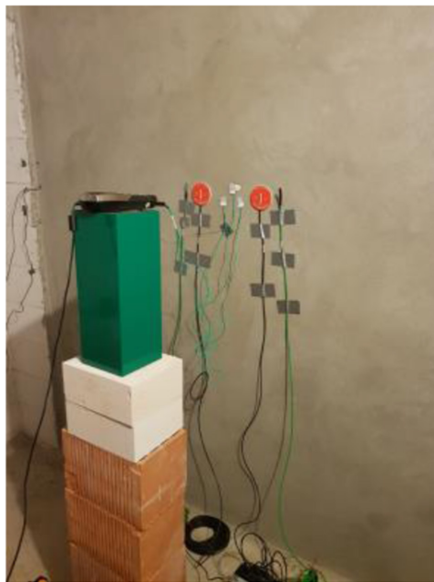
Figure 5: HFM method and TBM.
