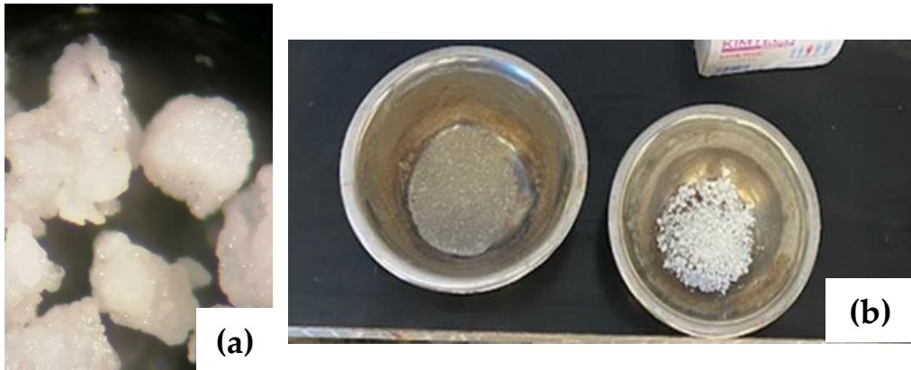
Figure 1. Appearance of: (a) TDI microcapsules (enlarged) and (b) crystalline hydrophilic additive (left) and TDI microcapsules (right)
