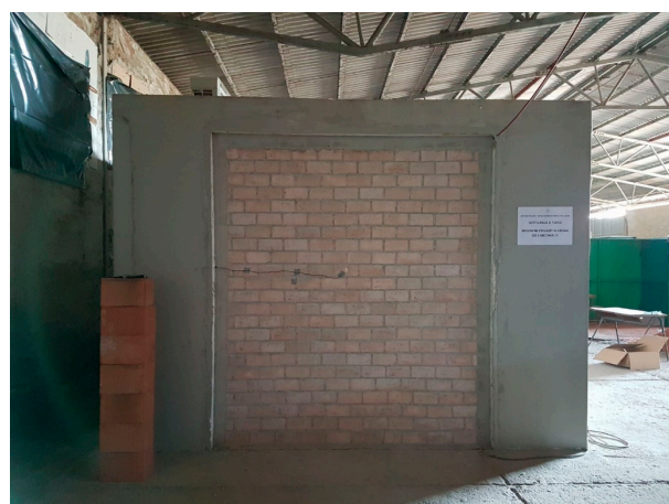
Figure 5. Wall made of RBC-EP masonry block—without isolation.
