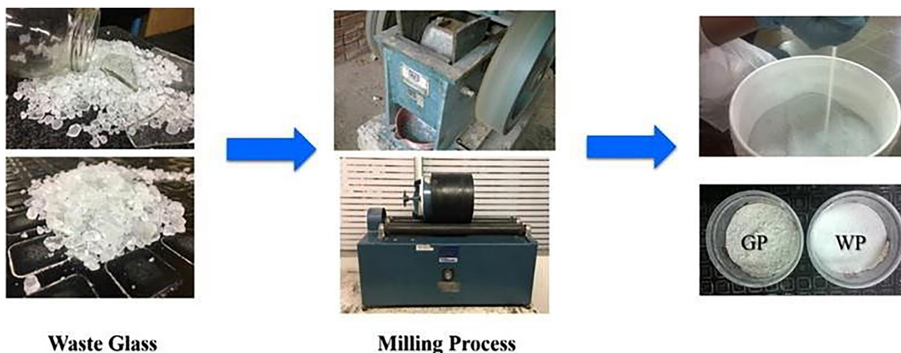
Fig. 1. Processing of glass wastes to GP (reused with permission (Rivera et al., 2018)).
