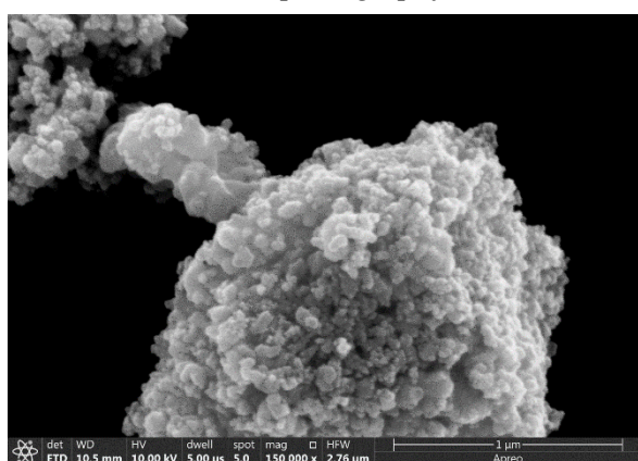
(g) SEM microphotography of \gamma -Fe 2 O 3
