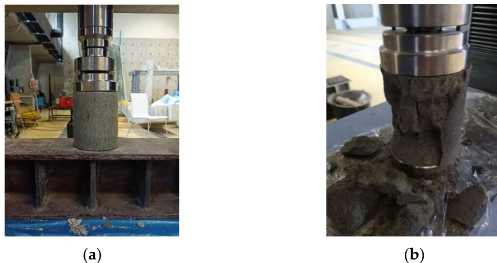
Figure 7. Compressive strength test: (a) before loading and (b) after loading.
