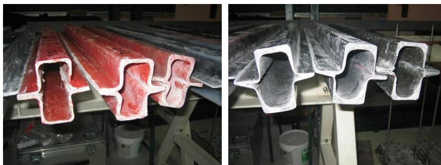
Figure 6. Testing beam samples from GFRP and RGFRP
