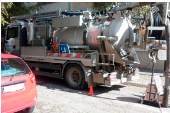
Figure 5. Sewer cleaning truck (Photo by D. Obradović).
