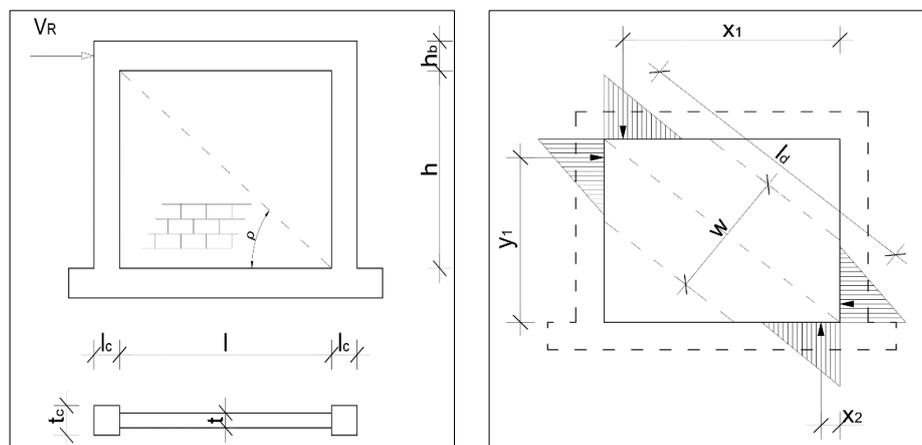
**Figure 7. (a) RC frame with a masonry infill wall scheme; (b) idealised compressive stresses in the wall corners (ends of the diagonal strut) [56]**
