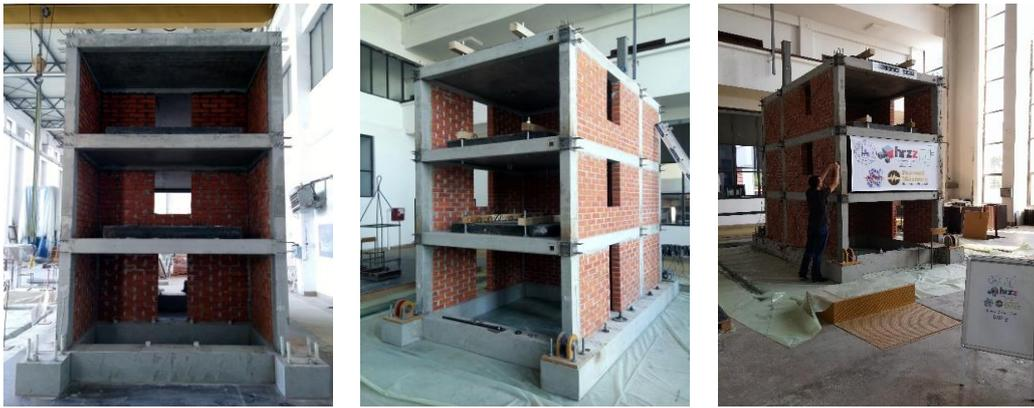
Figure 1. A view on the 1/2.5 scale three-story masonry infilled reinforced concrete frame building before testing
