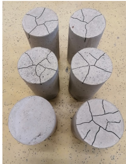
Figure 5. Mixture SCC-R—occurrence of cracks at the bottom of the specimens (400 °C and 600 °C).
