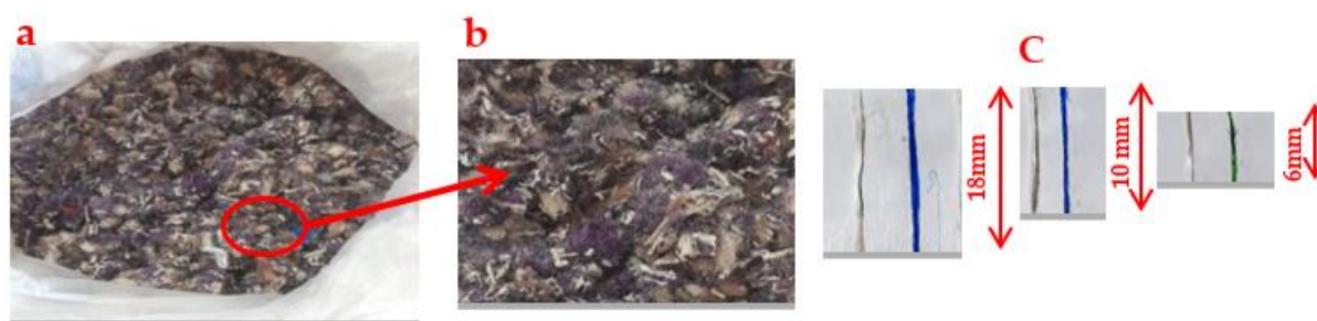
Figure 1. (a) Hybrid synthetic waste fibers; (b) enlarged image of hybrid synthetic waste fibers; (c) the size of the hybrid synthetic waste fibers.
