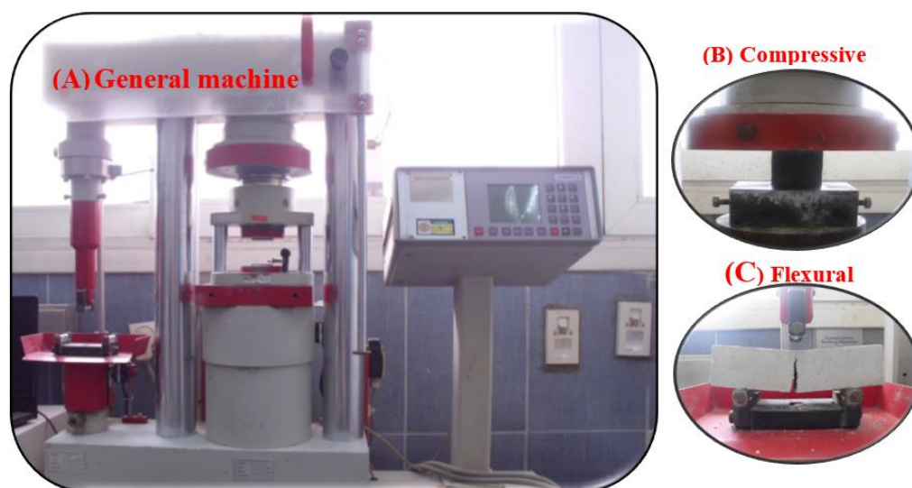
Figure 4. View of testing: (A) machine, (B) compressive strength, and (C) flexural strength.
