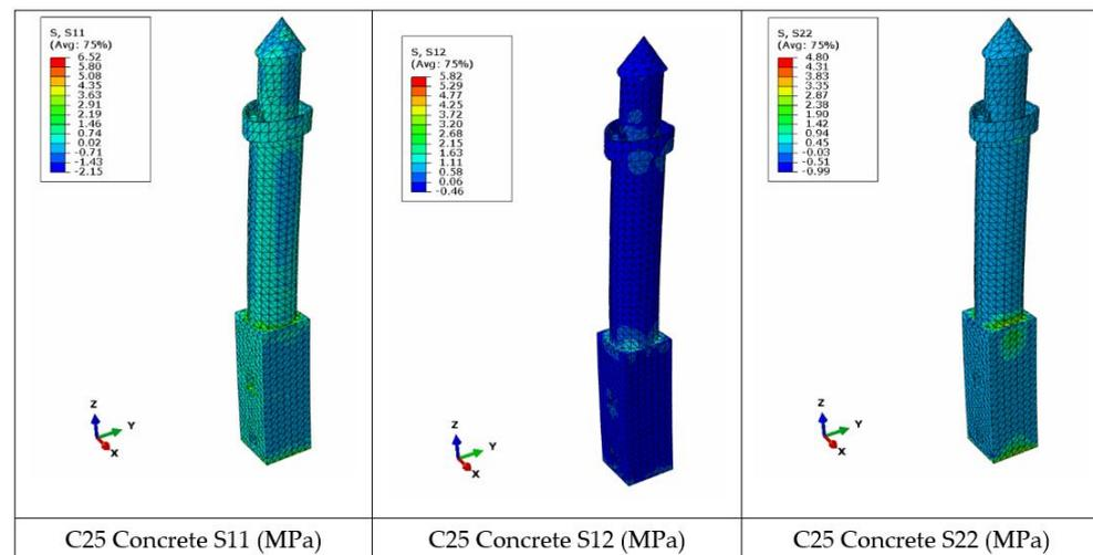
Figure 15. Stress diagrams for C25 concrete (H = 25.40 m).
