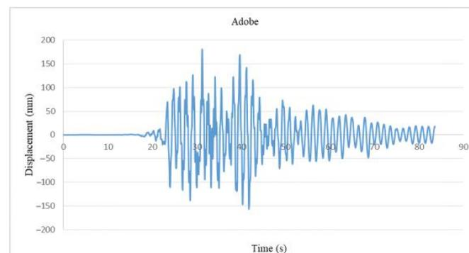
**Figure 18.** Time-displacement curve for minaret made of adobe.
