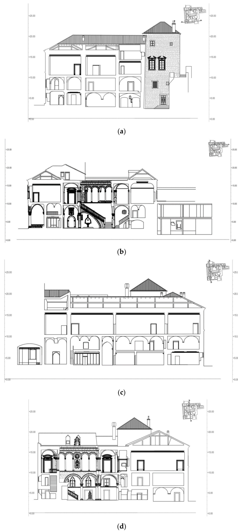
Figure 7. Selected cross-sections of the Rector's Palace: (a) "2-2"; (b) "3-3"; (c) "6-6"; (d) "9-9" as specified in original architectural drawings (courtesy of the Institute for the Restoration of Dubrovnik).
