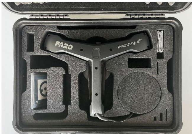
Slika 2. FARO Freestyle 3D laserski skener
