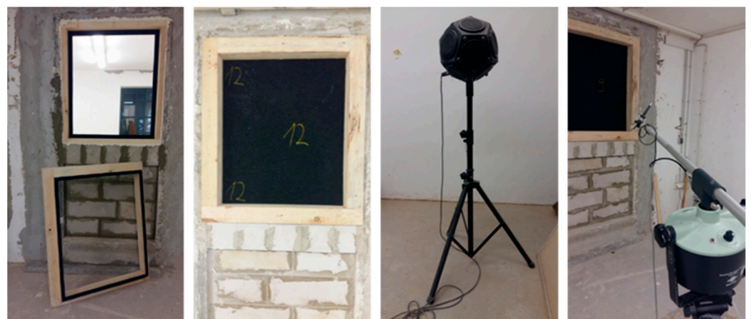
Figure 7. Airborne sound insulation index test setup.
