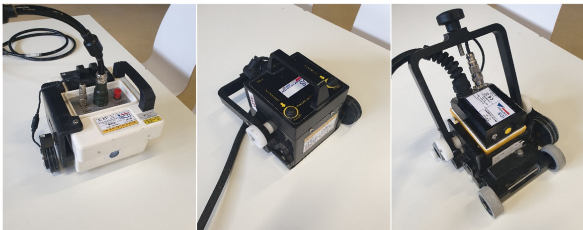
Figure 24. The test antennas: 900 MHz (left), 2.0 GHz (center), and 3.0 GHz (right).
